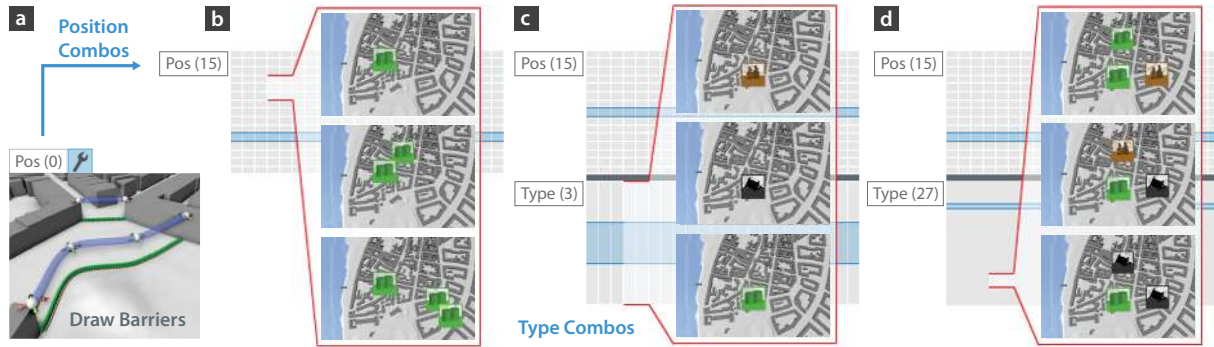
Figure 4: Combinatorial ensembles. (a) Based on multiple user sketches, the system (b) generates an ensemble of barrier positions containing all possible combinations, indicated in zoom lenses. (c) Added dimension for barrier types. (d) Depending on the selected position combination, a different number of type variations is possible and displayed.
