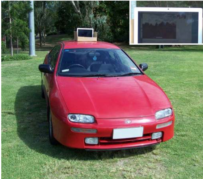
Fig. 5. Apple Macbook with built-in iSight video camera (inset) mounted on the test vehicle. This camera was the sole source of sensory information for the mapping system. The laptop was mounted on the roof of the car in a forward facing, zero pitch position.
