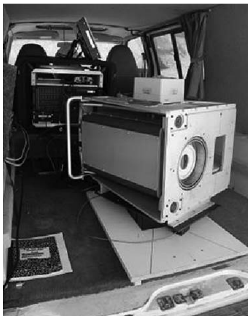
Figure 5. ProSpecTIR-VS scanner in custom configuration on rotating turntable in the vehicle for mine-wall (outcrop) scanning. The short-wave infrared (SWIR) instrument is on the left side of the box (round lens). The visible and near-infrared (VNIR) instrument is behind the rectangular port on the right.
