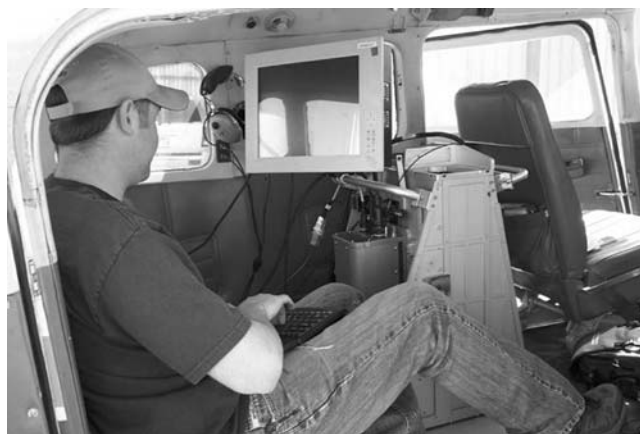
Figure 3. ProSpecTIR-VS hyperspectral scanner mounted in Cessna 206 aircraft.
