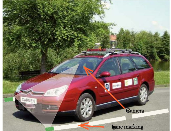
Fig. 5. Experimental vehicle. The camera is located behind the windscreen.
