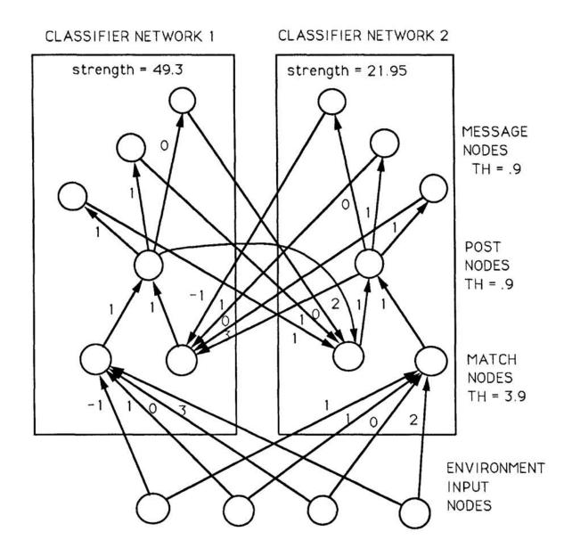
Figure 1: Result of mapping a classifier system with two classifiers into a neural network. Classifier 1 has match field (0 1 #), message field (1 1 0), and strength 49.3. Classifier 2 has match field (1 1 #), message field (0 1 1), and strength 21.95.
