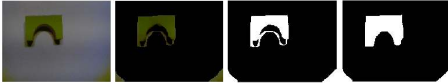
Figure 5: Image processing - original image, removal of the background, converting to BW image and filling the holes
