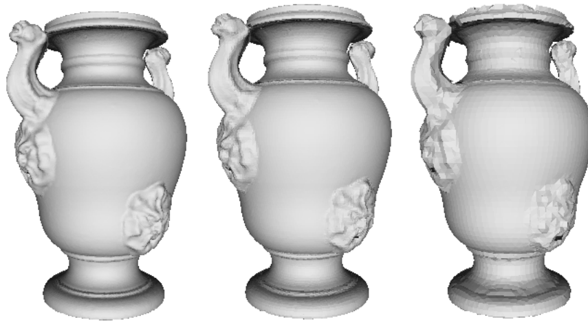
Figure 7. Three decimated levels of the Vase model (originally, 2,104,096 triangles): 523,052, 109,912, and 22,782 triangles for the left, center, and right image, respectively.
