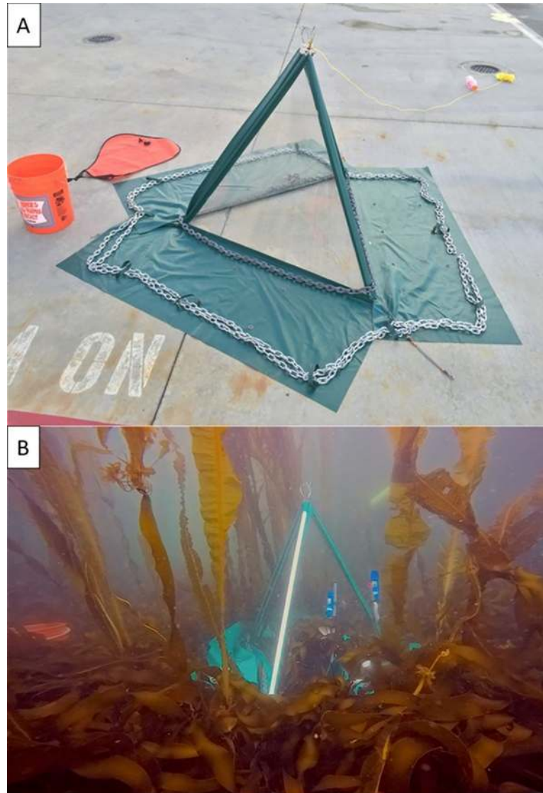
Fig 8. Photograph of cBIT. Photograph of (A) cBIT before deployment showing 26" skirt around perimeter, flexible polycarbonate walls, steel framing, anchor chain used to hold skirt and cBIT to the benthos, and (B) cBIT deployed in kelp forest showing PAR and oxygen sensors placed both inside and outside the chamber.
