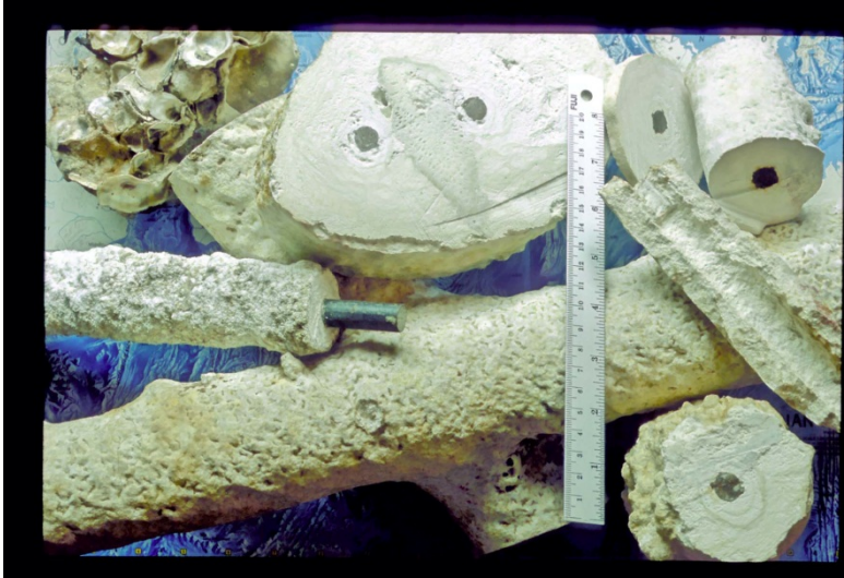
Figure 2. Bio-rock materials from various locations. The piece at mid left is the one shown in the previous photo. The one at top left, completely overgrown with oysters, is from Louisiana, and all the rest were grown in a two and a half year period at Ihuru Island, North Male Atoll, Maldives. Samples tested from that set of samples in the Materials Testing Laboratory of the University of Graz, Austria, had compressive strength of 60-80 Mega Pascals, around three times the load bearing strength of ordinary Portland Cement concrete. Photograph Wolf W. Hilbertz.
