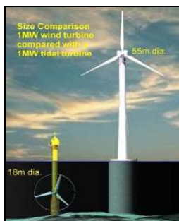
Fig. 5. Tidal turbine against an offshore wind turbine [© MCT].
