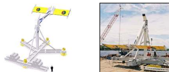
(a) The Stingray turbine. (b) Deployment for submerged testing.
