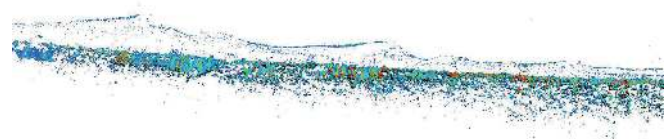
Fig.13. MarLS visualization for the coast fragment with the cloud density parameter of approximately 30 points per m2 for the green colour to approximately 100 points per m2 for the red colour
