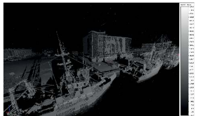
Fig. 12. MarLS visualization for vessels in harbour and port infrastructure (Laser data – number of points per square meter)
