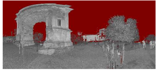
Figure 7: Outdoor environment with Roman arch, paths, vegetation, and a distant building. Note the numerous artefacts caused by walking people.
