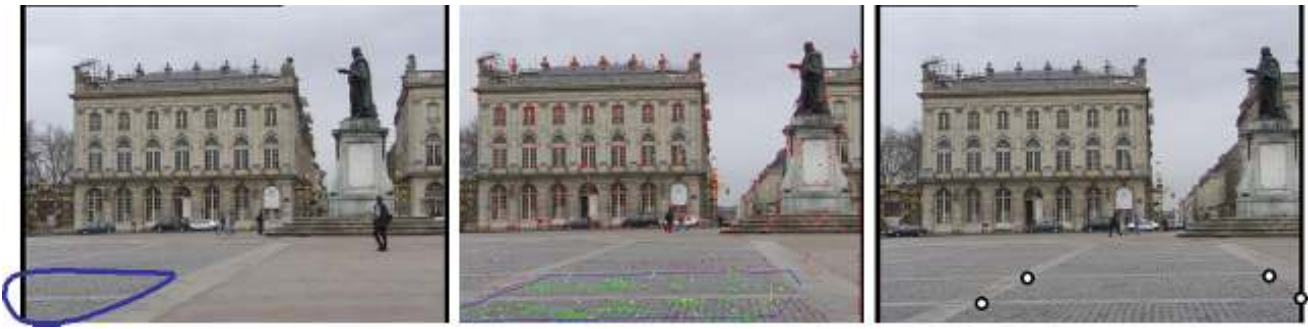
Figure 4. Steps in the algorithm. (1) The plane to be tracked is roughly indicated with the mouse, with the camera stationary. (2) Automatic feature detection and tracking. (3) Setting the coordinate system by indicating 4 points on a rectangle. At no point after (1) need the camera be stationary, nor tracking interrupted.
