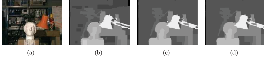
Figure 11: Comparison of different optimization algorithms. (a) image is the original left image. (b) is the result BP. (c) is the result by \alpha -expansion. (d) is the result TRW [44].
