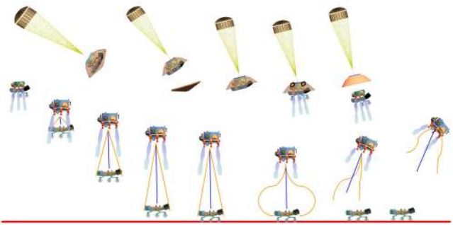
Figure 9: MSL’s skycrane descent sequence.
