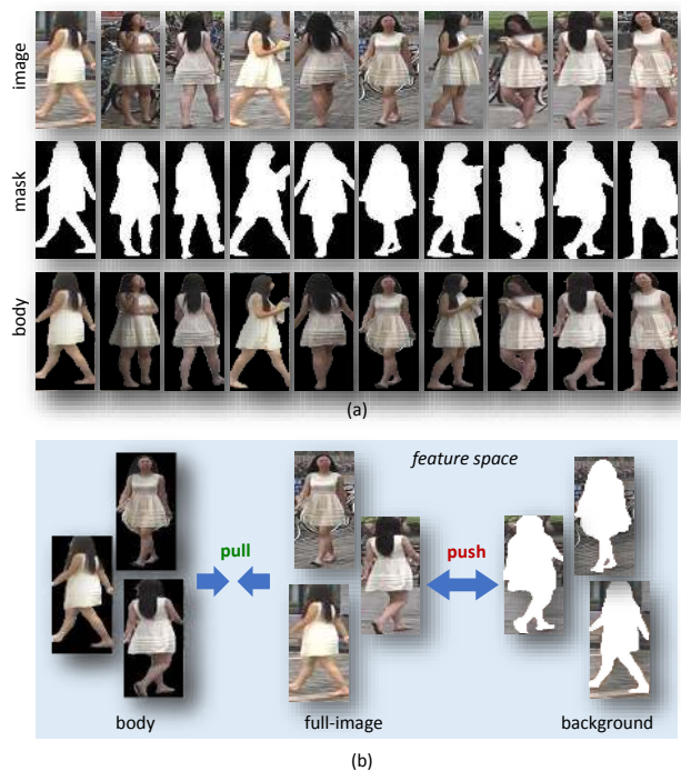
Figure 1. Illustration of the binary mask and region-level triplet loss for contrastive feature learning. (a) Examples of RGB images and their corresponding masks. The third row shows the body regions extracted directly with the masks. (b) The proposed region-level triplet loss can restrain the features learnt from different regions, i.e., pulling the features from the full image and body region close, whereas pushing the features from backgrounds away.
