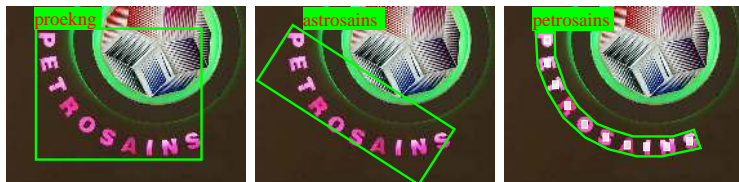
Fig. 1: Illustrations of different text spotting methods. The left presents horizontal text spotting methods [30, 27]; The middle indicates oriented text spotting methods [3]; The right is our proposed method. Green bounding box: detection result; Red text in green background: recognition result.
