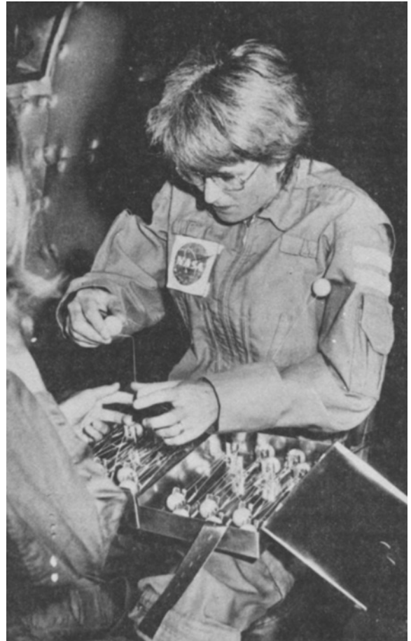
Figure 4. Preliminary version of the mass-discrimination apparatus in use during parabolic flight.
