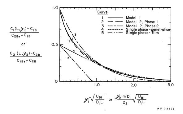
Fig. 7. Effluent concentrations; comparison of models. R = 1.
