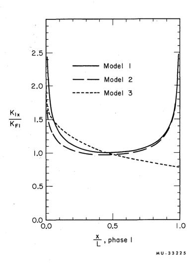
Fig. 4. Local mass transfer rates; comparison of models. R = 1.
