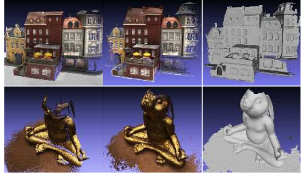
Figure 5: Reconstruction results of two DTU objects. From left to right: ground truth point cloud, textured point cloud and triangulated mesh surface.
