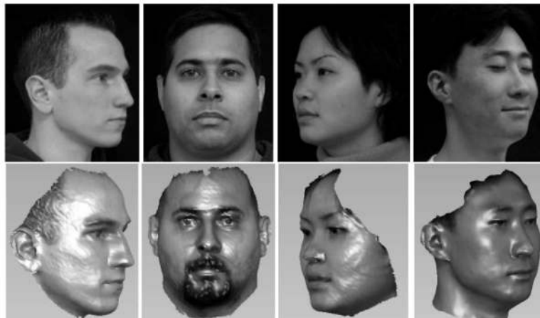
Fig. 17. Test scans (top row), and the corresponding 3D models correctly matched. The 3D model is shown in a pose similar to the corresponding test scan.
