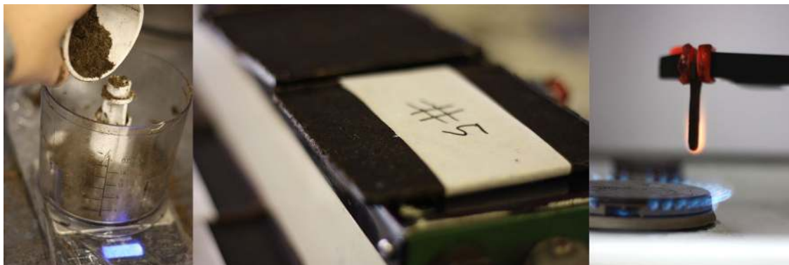
Figure 2. Tinkering with the material: varying the amount of coffee grounds in different samples to be subjected to mechanical tests (left and middle); fire resistance test (right).
