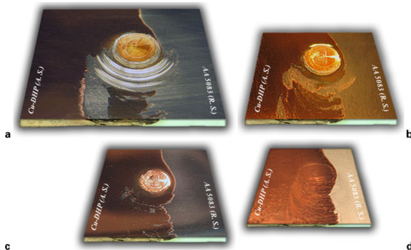
10 Horizontal cross-sections of C-1000_16_Cu weld at a 0.74 mm, b 0.66 mm, c 0.61 mm and d 0.41 mm from root
