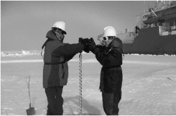
Fig. 5 Augering for ice thickness measurement
