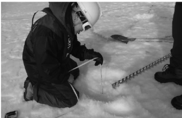
Fig. 6 Thickness measurement using ice gauge
