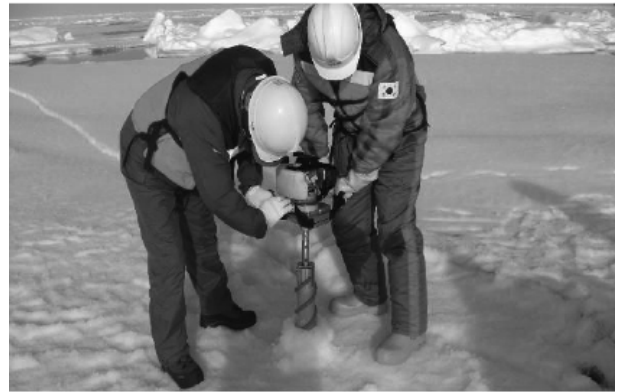
Fig. 7 Coring with 3" ice corer
