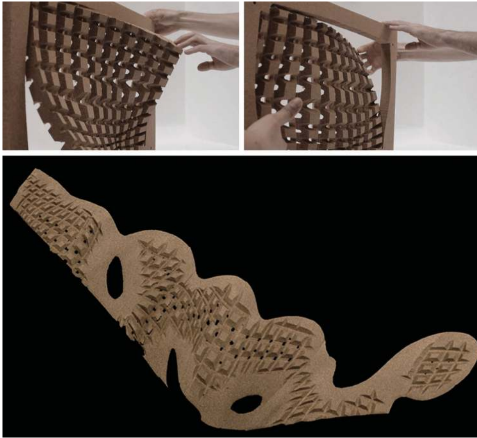
Figure 2. Cork gains intended flexibility and double-curved bending.
