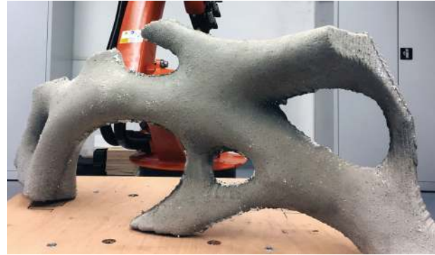
Figure 5. Concrete branch test sample, with robotically produced mound with two temporary mould parts.
