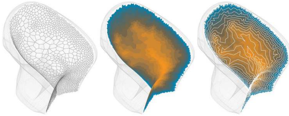
Figure 20. Resulting cell distribution after human body analysis (left); toolpath optimization following a radial logic (middle); continuous toolpath travels through all cells without hovering above the surface (right).
