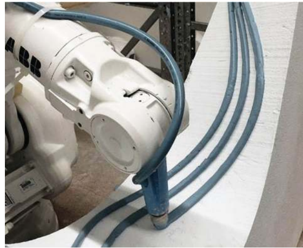
Figure 10. Robotic 3D printing on a freeform surface.
