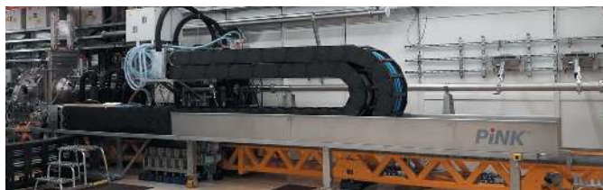
Figure 8 Photograph of the SAXS configuration where the bellows between MPC and AGIPD are fully compressed reducing the sample-to-detector distance to \sim 3 m.
