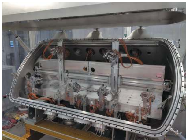
Figure 3 Photograph of the open split-delay line installed in MID's OH with the mechanics and optics inside visible.
