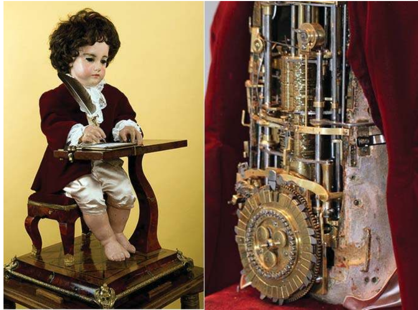
Figure 1: An automaton: a device called “The Writer”, built in the 1770s by a Swiss watchmaker, Pierre Jaquet-Droz (1721-1790), and his family: son Henri-Louis Jaquet-Droz and Jean-Frédéric. This automaton could write sequence of letters composed thanks the the mechanical interface on the back of the doll [50].
