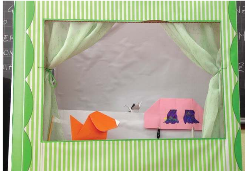
Figure 48: This picture has been taken during the demo of the story the researchers created to show how the smart origami models worked with the story. From the left: 1) in orange, the barking dog, actuated by a NiTiNOL wire, 2) in the centre a crane with thermochromic ink on the wings and 3) on the right, a house with flowers hidden behind the thermochromic curtains of the windows. On the outside, in green, one of the cardboard theatres also used during the children's presentations.
