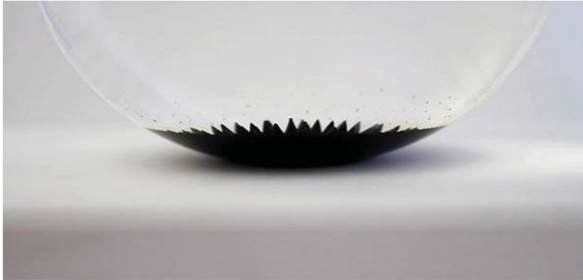
Figure 4: Magnetic Mind is a project that translates brainwaves into kinetic art, using a NeuroSky MindWave brain-computer interface headset, an Arduino, an electromagnet and suspended ferrofluid.
