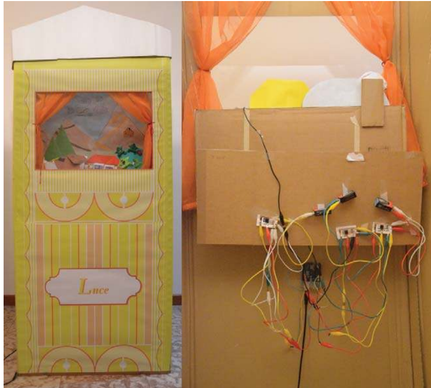
Figure 52: The cardboard theatre: front-end and backstage. On the right it is possible to see all the component to control the actuations. Arduino is the element on the bottom, in the middle there are the control switches and just over them the battery to power the animations.
