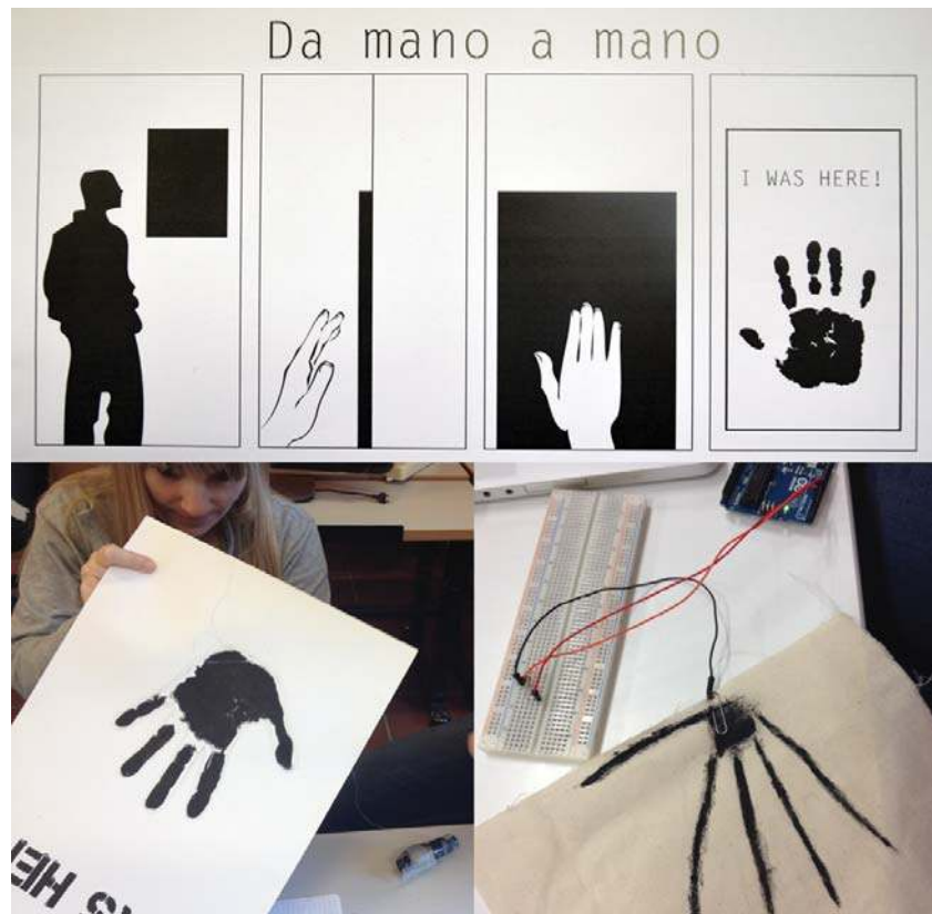
Figure 57: Development of project Da mano a mano , from the students' sketches. On the top the concept design and on the bottom picture of the aesthetics and the capacitive hand sensor drawn with conductive ink.
