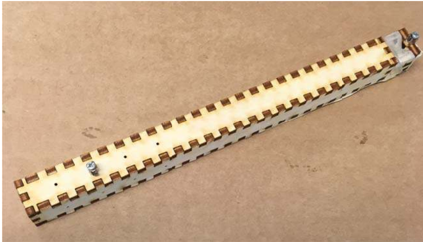
Figure 59: The root actuator, final version, is catted from a plate of 3mm poplar wood, the operation of cutting require about 3 minutes, and so the assembly. The silicon spring is casted from a batch mould made of perspex also laser cut. The total size is comparable the older one. The hinge mechanism is still made of tape (perfectly functional, cheap and easy to connect).
