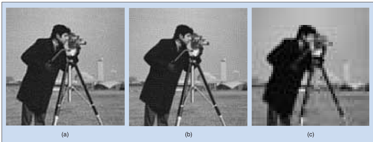
▲ 11. Reconstructed images using (a) the model in (2) [relative error = 0.0614], (b) the joint minimization model with the H^1 -norm regularization [relative error = 0.0574], and (c) the joint minimization model with the total variation regularization [relative error = 0.0931].
