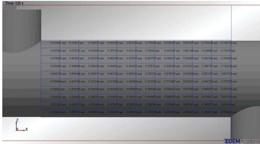
FIGURE 2: EDEM snapshot showing radial powder velocities in the mixer at time t = 120 s.
