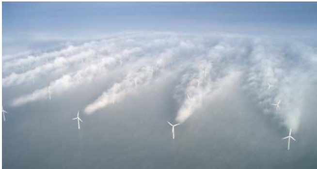
Fig. 1 Wake effect in an offshore wind park [Vattenfall]
