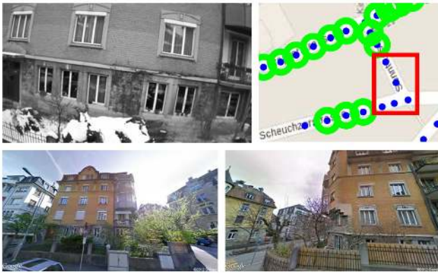
Fig. 9: Analysis of the first false-positive detection. Top-left: urban MAV image; top-right: zoom on the global map, where the image was taken; bottom-left: detected match; bottom-right: true positive pairing according to manual labeling. Please note that our algorithm fails for the first time in a situation where the MAV is facing the same building from two different sides (streets), having in the field of view only windows with the same patterns.
