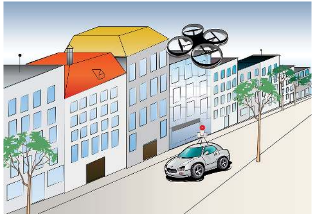
Fig. 1: Illustration of the problem addressed by this work. The global position of the MAV is computed by matching the aerial image taken by the flying vehicle with the closest ground-level geotagged Google Street View image.
