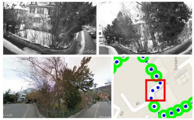
Fig. 10: Analysis in case of no detections. Top-left: urban MAV image; top-right: next view of the urban MAV; bottom-left: true positive pairing according to manual labeling; bottom-right: zoom on the global map, where the image was taken. Please note that these robot positions (top row) are difficult to be recognized even for humans. Moreover the over-season change of the vegetation makes it extremely difficult to cope with the pairing of them for image feature based techniques.
