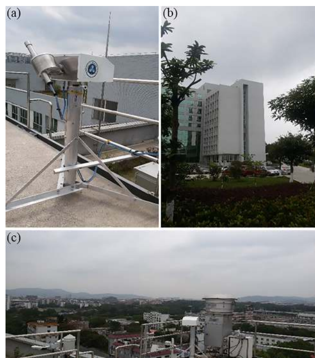
Figure 1. The tracker and entrance optics of the Phaethon MAX-DOAS system (a) installed on the roof of the Institute of Geochemistry, Chinese Academy of Sciences, in Guangzhou (b) and an overview of the surrounding area towards west (c).
