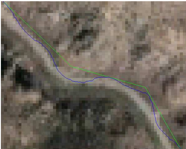
Fig. 15. Results from the second flight through Goshen Canyon. Flight test results show the planned path (green) and the actual path (blue). The planned path was intentionally biased to the east forcing the MAV to offset from its planned path to center itself through the canyon.
