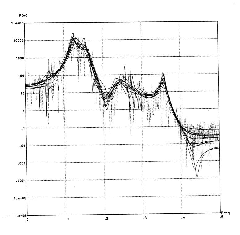
Figure 9.3c - Colored Gaussian Noise, AR(50) Based MEM(12,8) Model (solid), Periodogram (dotted)
