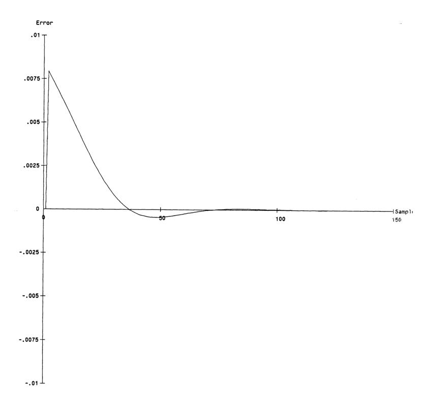
Figure 7.1 - Error Between Impulse Response Coefficients of MEM(0,1) and AR(500) Models
