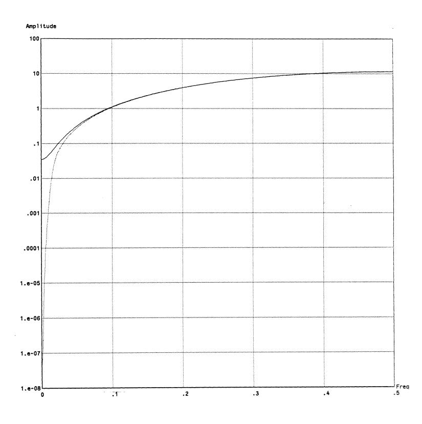
Figure 7.3 - Power Spectra of MEM(0,1) (solid) and AR(500) (dotted) Models
