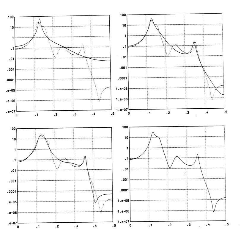
Figure 9.1 - MEM(4,0), MEM(6,2), MEM(8,2), MEM(8,4) (solid) and original spectrum (dotted)
