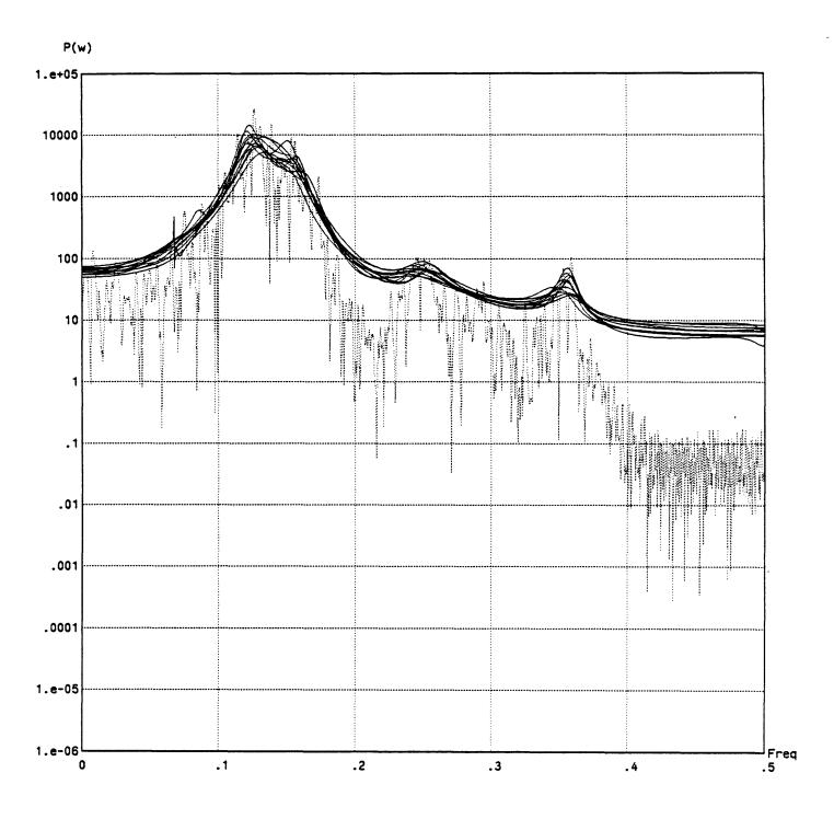
Figure 9.3b - Colored Gaussian Noise, Triangular Window Based MEM(12,8) Model (solid), Periodogram (dotted)
