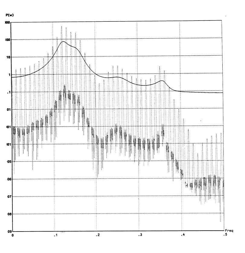
Figure 9.2b - Impulse Train Excited Filter, Triangular Window Based MEM(10,6) Model (solid), Periodogram (dotted)
