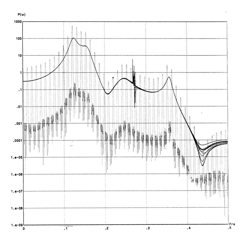
Figure 9.2c - Impulse Train Excited Filter, AR(50) Based MEM(10,6) Model (solid), Periodogram (dotted)
