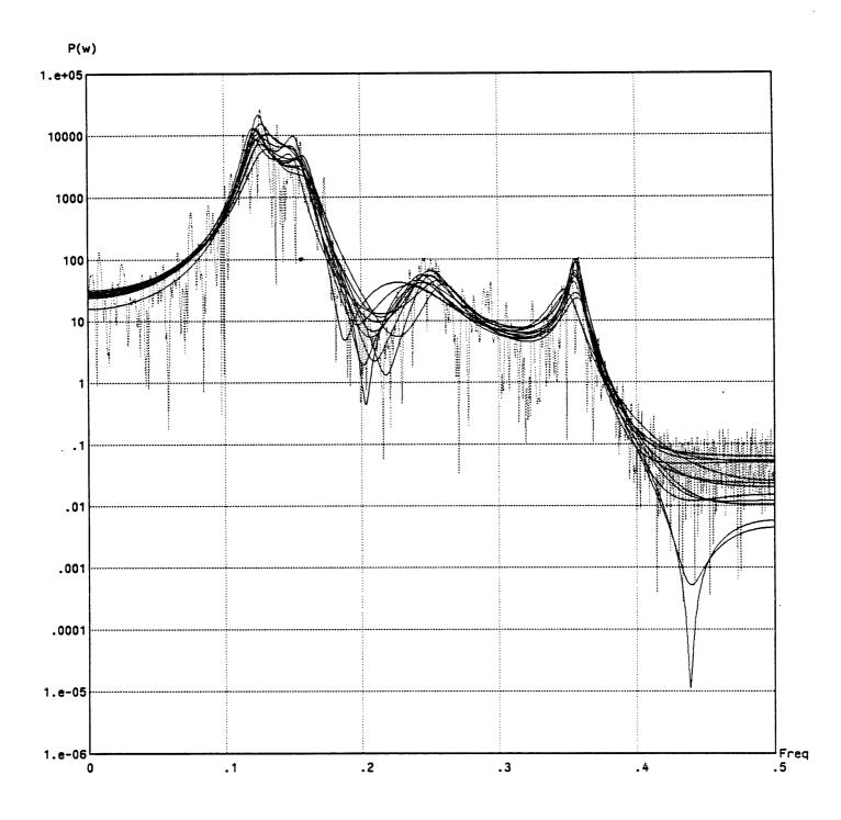
Figure 9.3d - Colored Gaussian Noise, AR(40) Based MEM(8,4) Model (solid), Periodogram (dotted)
