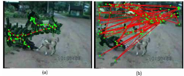
Figure 5. The trajectories of centroids of selected regions, green dots connected with red lines, overlaid over the first frame: (a) when inter-frame mutex constraints are used and (b) when inter-frame mutex constraints are not used.
