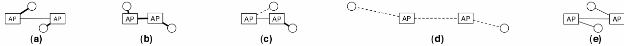
Figure 8: Case (a): AP-client link is strong ( > -55 dBm) and AP-AP link is weaker by at least k dBm. Case (b): AP-client and AP-AP links are strong ( > -55 dBm); they only increase their CCA. Case (c): AP-client link weaker than AP-AP link; PC cannot shrink cells. Case (d): AP-client links are quite poor; no reduction in power or increment in CCA is possible. Case (e): AP-client links not much stronger than AP-AP links; isolation is impossible.
