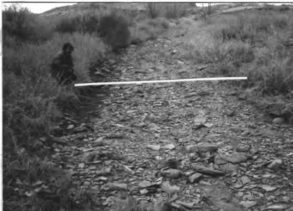
Figure 4.--Active-channel section on Spring Creek near Decker, Montana. Section is defined by vegetation and change in slope; width is about 13 feet. Site is near station 06306900. View is upstream.
