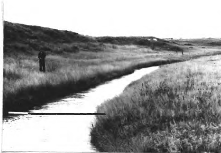
Figure 6.--Active-channel section on North Fork Coal Bank Creek near Mill Iron, Montana. Section is defined by vegetation and change in slope; width is about 14 feet. Site is at station 06334640. View is downstream.
