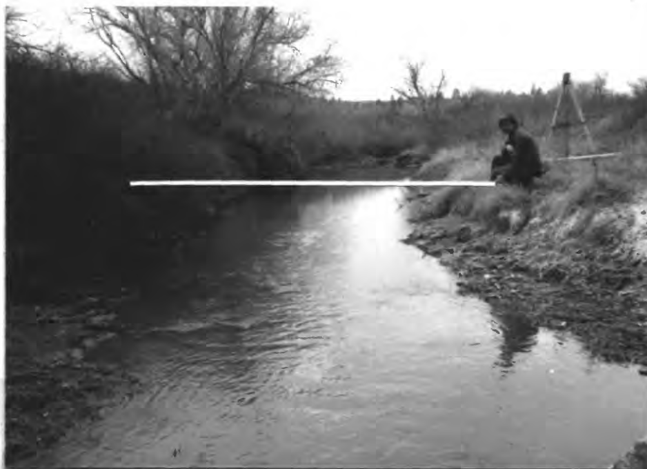
Figure 7.--Bankfull section on Tullock Creek near Bighorn, Montana. Section is defined by change in slope between bank and flood plain; width is about 25 feet. Site is near station 06294690. View is downstream.
