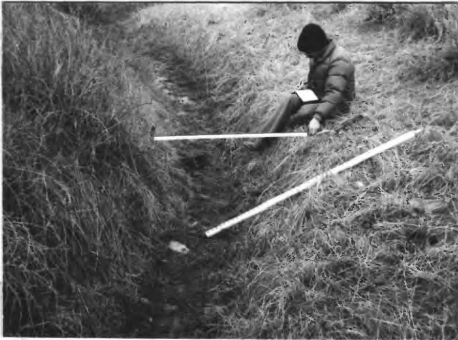
Figure 8.--Bankfull section on Pearson Creek near Decker, Montana. Section is defined by change in slope; width is about 4 feet. Site is near station 1. View is upstream.
