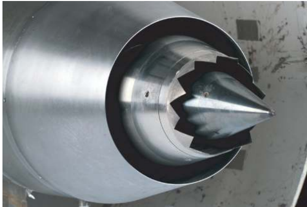
Figure 1.—Separate flow nozzle 3A 12 B hardware.
