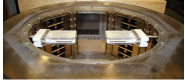
FIGURE 3: View of the measurement tank with the two sensors (Cassiopeia antenna) attached to movable arms.
