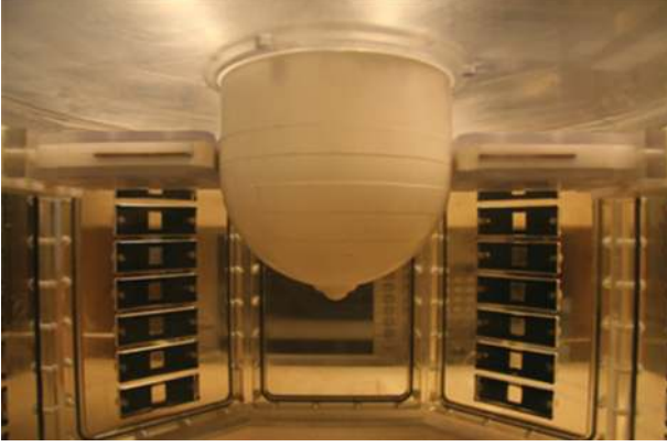
FIGURE 5: View of the low-loss breast model in the measurement tank. Picture was taken without the 2% saline for better clarity.
