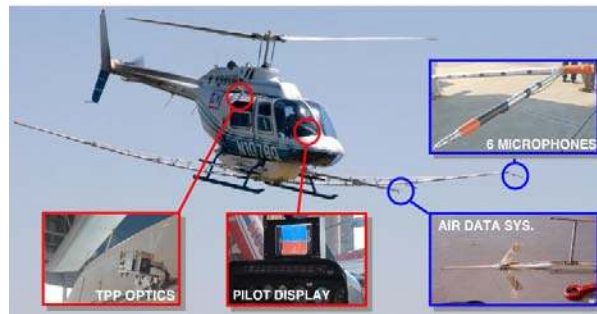
Figure 3: In-Flight Boom Mounted Microphone System, Air Data Boom, Pilot Display and TPP Measurement Optical System
