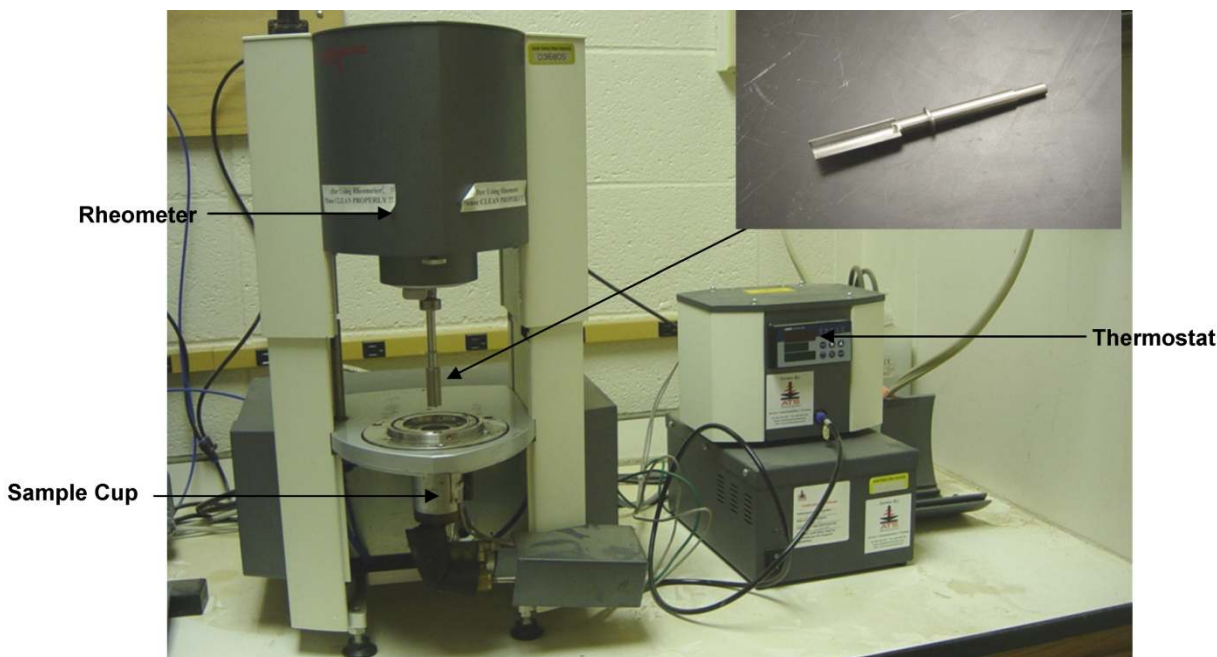
Fig. 2. Experimental setup used to measure the sticky point temperature ( T_s , ^\circ\text{C} ) using a rheometer. The four-blade vane stirring tool (36.79 mm in length, 6.78 mm in width, and propeller shaft 105.63 mm in length) is enlarged in the inset.
