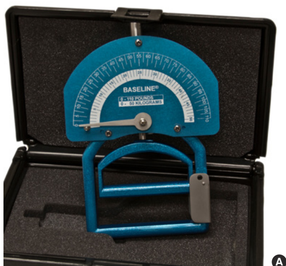
Fig. 3. Mechanical type dynamometer (Smedley type). (A) Baseline. (B) Takei, GRIP-A.
