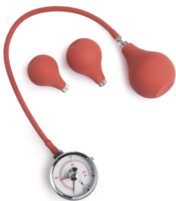
Fig. 2. Pneumatic type dynamometer (Martin Vigorimeter). Three sizes of balloons are available for pediatric and adults.
