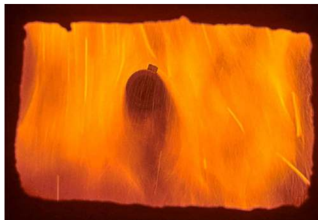
Figure 11. Picture of the coal flame during measurements with the optical probe without the water-cooled beamstop. The photo is taken through the quartz window, used as a cold background, at the opposite side from where the probe was inserted. In the photo, the probe tip is approximately in the center of the flame.
