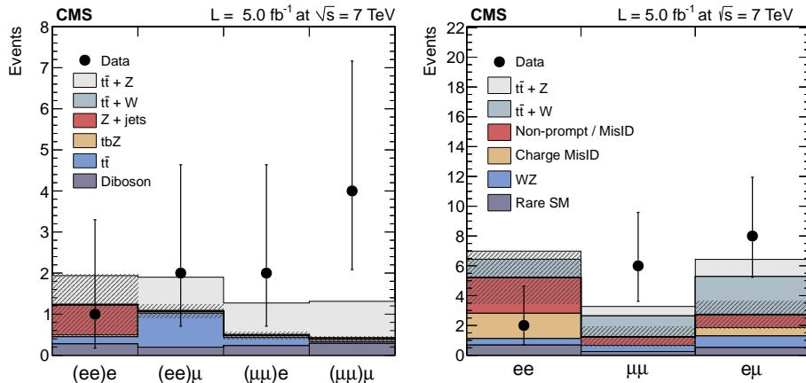
Figure 2: Event yields after final selection requirements, separated in lepton flavor channels for the trilepton (left) and same-sign dilepton (right) analyses. The expected contributions from signal and background processes are shown, and the uncertainty on the estimated background yield is superimposed with a grey hashed band.
