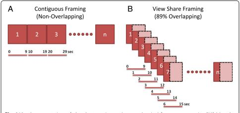
**Fig. 1** Visual representations of ultra-short contiguous (non-overlapping) frame reconstruction [11] (**a**) and view-sharing (89 % overlapping) frame reconstruction (**b**) used with stationary and rotating gantry PET systems, respectively
