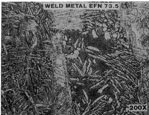
Fig. 17 Microstructure of Ferralium 255 SMA Weld Metal, FN 73.5, 200 X, Kallings Reagent.
