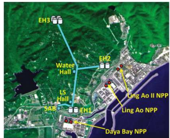
FIG. 1. Layout of the Daya Bay experiment. The Daya Bay and Ling Ao nuclear power plant (NPP) reactors (red circles) were situated on a narrow coastal shelf between the Daya Bay coastline and inland mountains. Two antineutrino detectors installed in each underground experimental hall near to the reactors (EH1 and EH2) measured the \bar{\nu}_e flux emitted by the reactors, while four detectors in the far experimental hall (EH3) measured a deficit in the \bar{\nu}_e flux due to oscillation. The detectors were built and initially tested in a surface assembly building (SAB), transported to a liquid scintillator hall (LS Hall) for filling, and then installed in an experimental hall.
