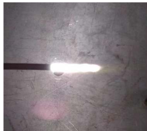
FIG. 2. Photo of a torch supported by focused microwave radiation from. Electromagnetic wave propagates from left to right. Exposure time 0.1 s.
