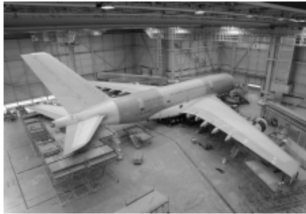
Fig. 5. Ground vibration tests on Airbus A380-800 (copyright Airbus S.A.S.).
