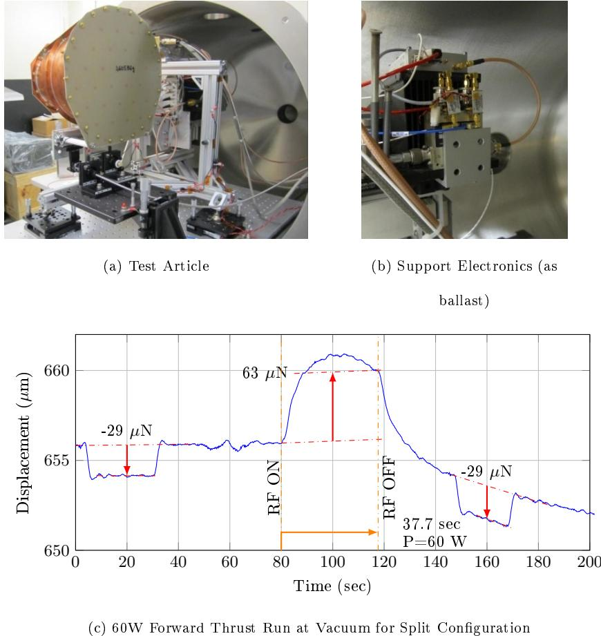
Fig. 10: Split Configuration: The pictures show how the pendulum arm was loaded with the test article on one end, and the support electronics on the opposite end serving as ballast. The thrust trace illustrates the quicker rise times for the pendulum in response to an impulsive signal.
