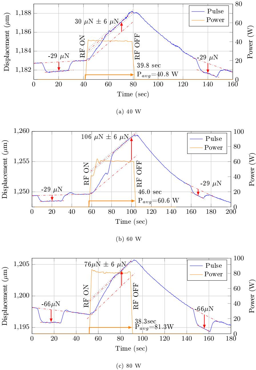
Fig. 13: Forward Thrust, at Vacuum, Representative Runs. Error bars ( $\pm 6 \mu\text{N}$ ) are shown as black dotted lines.
