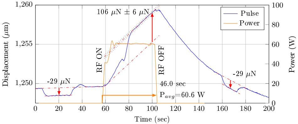
Fig. 7: Superposition of Signals: Test Article Run at 60 W in Vacuum.
