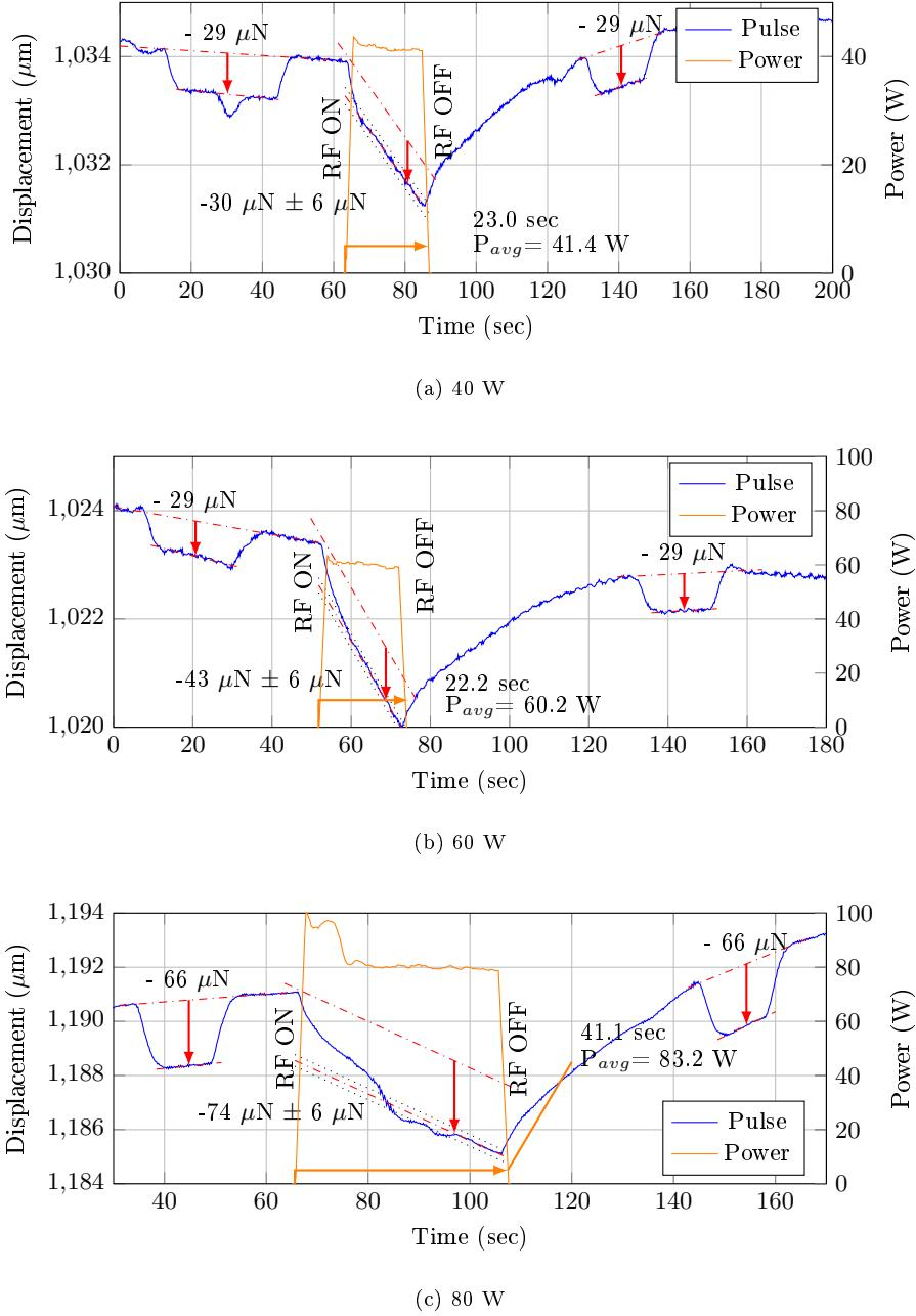
Fig. 16: Reverse Thrust, at Vacuum, Representative Runs. Error bars ( $\pm 6 \mu\text{N}$ ) are shown as black dotted lines.
